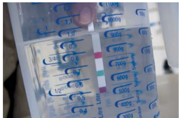
Test strips change in color (from white to purple) when chlorine contents are higher than 1 p.p.m.
